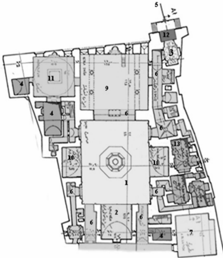
Fig. 3. The Vocabulary Elements of the Plan of al-Thaher Barquq madrasa, Cairo: 1– Courtyard (or dorqa'a ); 2–North-Western Iwan (opposite to Qibla Iwan); 3–Derka “entrance spaces”; 4–Small Cells for the Students; 5–Main Entrance and portal space; 6–Corridors and Transitional Spaces; 7–Ablution Space; 8–Sabil (free water fountain); 9–South-Eastern Iwan (Qibla Iwan); 10–Southwestern and Northeastern Iwans ; 11–Tomb or Mausoleum for the madrasa’s patron; 12–Minaret (see fig. 4); 13–Teacher’s House (Sheikh’s House); 14–Northern and Southern secondary Iwans ( Sadla ). (Reproduced by authors, from [Organization of Islamic Capitals and Cities 1990])
